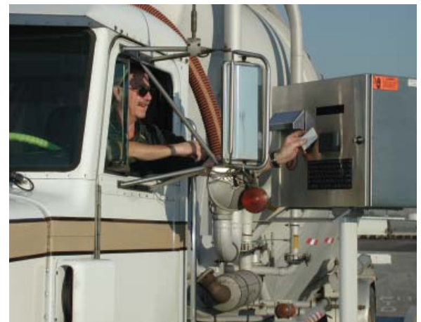
Unattended driver terminals keep traffic moving over scales by allowing drivers to process their own transactions in seconds.
