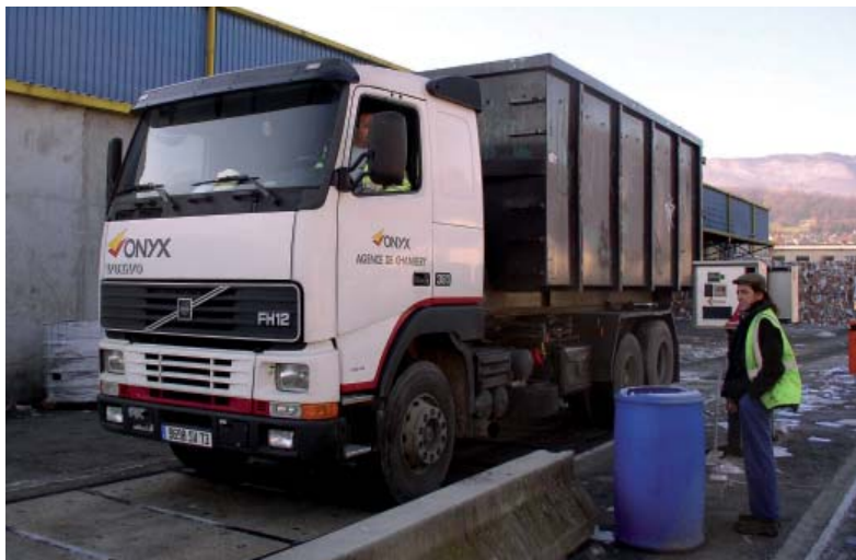
The new truck scale, unattended weighing terminals, and OverDrive software have significantly reduced the time needed to weigh trucks.
